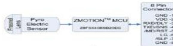
Figure 1: ZMOTION™ Block Diagram
